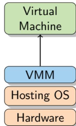
(b) *Type II or hosted VMM.* The VMM runs on top of a conventional operating system and uses OS services.
