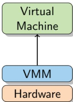
(a) *Type I, native or bare metal VMM.* Runs directly on the hardware in the most privileged processor mode.
